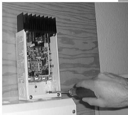
Figure 2-3 Mounting the C-Series Multifunction DC Controller
