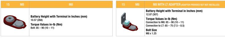
C. D. Height taken from bottom of the battery to the highest point on the battery. Heights may vary depending on type of terminal.
