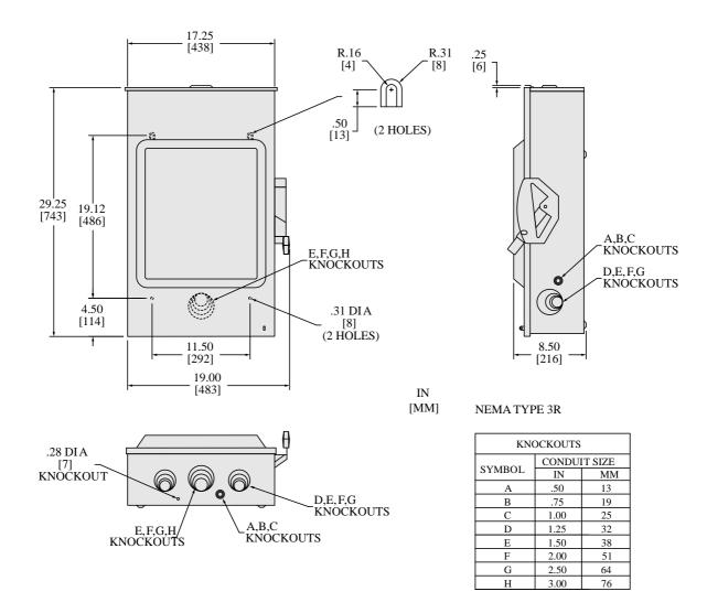
WHEN MOUNTING THESE SWITCHES, ALLOW  $4.00\ [102]$  MIN CLEARANCE BETWEEN ENCLOSURES FOR OPENING OF SIDE HINGED DOOR.
