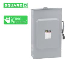
Safety switch, general duty, non fusible, 200A, 3 poles, 60 hp, 240 VAC, NEMA 3R, bolt-on provision
