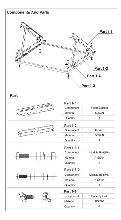
Assemble the components and parts together according to the left picture. Attached the PV module to the mounting brackets using M8 screw/bolt supplied in the pack. Be carful of the bolt, flat washer, spring wash and nut sequences. Find suitable holes on the panel frame and tighten the brackets on it.
