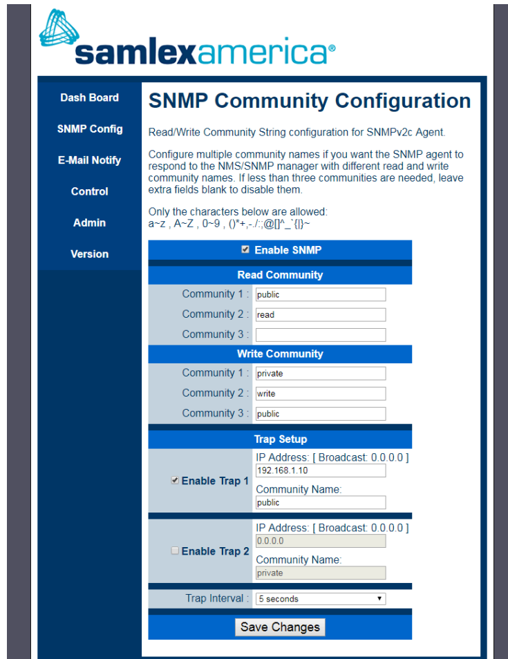
Fig 13.8 SNMP Community Configuration
