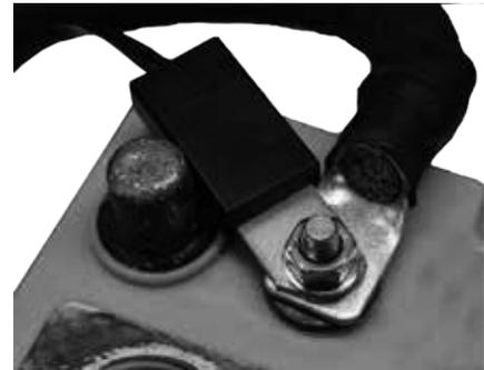
**Fig 2.5(b) Temperature Sensor Installation**
