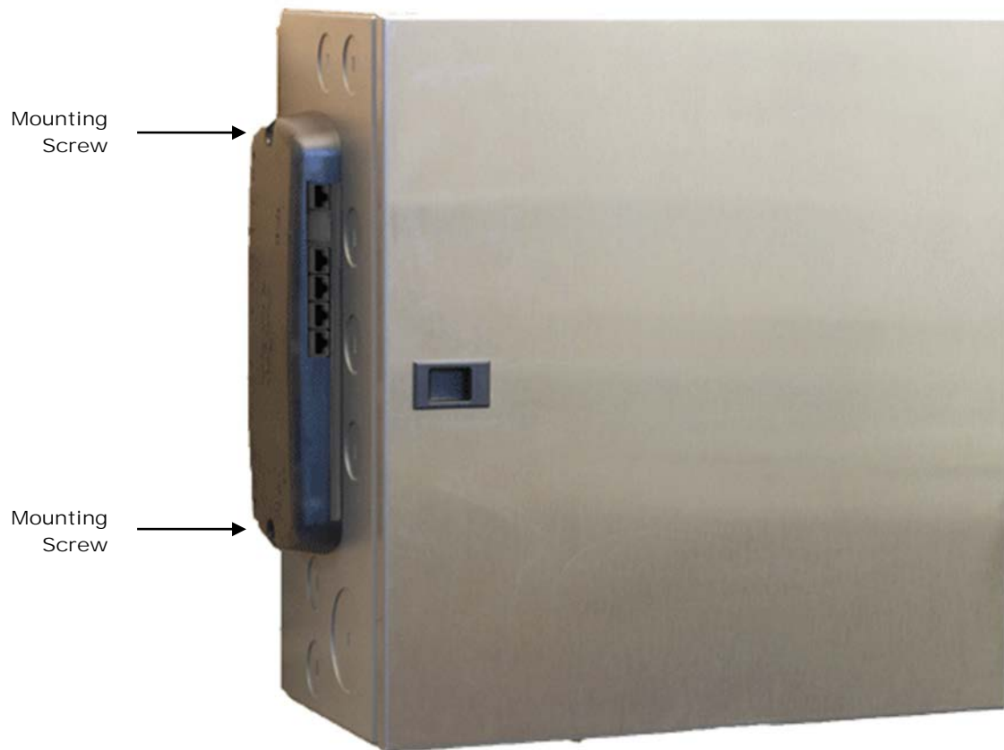
Figure 25 Mounting the HUB Product to the GSLC Enclosure
