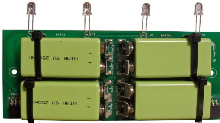
Battery – LED Board detail.
