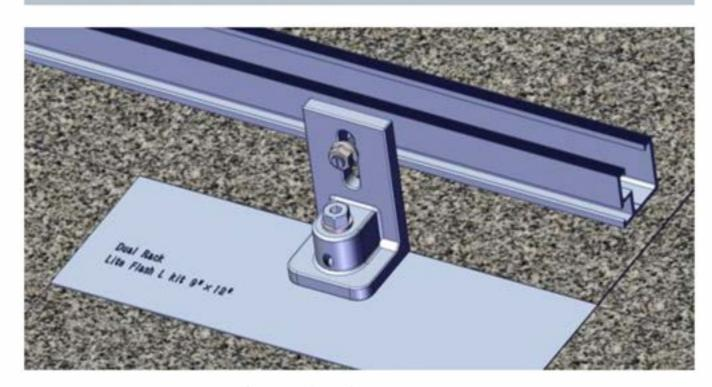
After locating and securely installing standoff to rafter, attach L=foot with 3/8" bolt and nut to Lite Rail at desired height.
