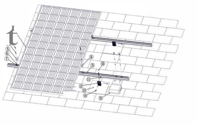
After locating and securely installing Flash L-Kit to rafter attach 3/8" bolt and nut to Lite Rail at desired height.
